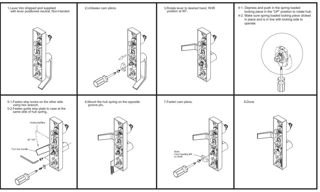
Method for replacing cylinder.
